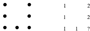
Fig. 3.5 Labeling of clusters for site percolation on a square lattice. The question mark shows the ‘conflict’ which arises in a simple labeling scheme.
